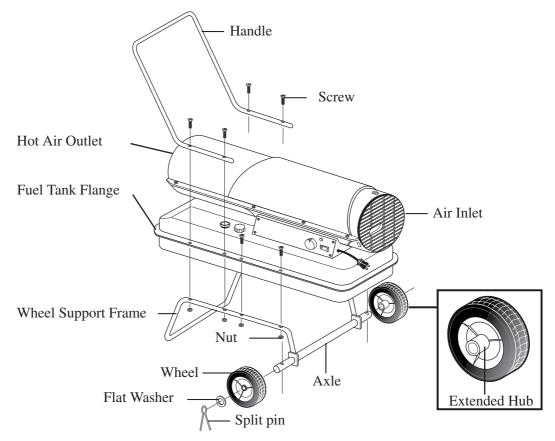
Figure 7. Wheel and Handle Assembly, RMC-KFA120T/RMC-KFA170T/RMC-KFA210T MODELS ONLY **NOTE:** Heater should be inspected before each use, and at least annually by a qualitied service person.
